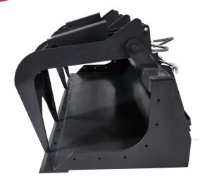
The Skid Steer Grapple Bucket functions the same as Arrow Skid Steer Buckets with the addition of grapple arms. The Grapple Bucket is great for moving scrap, logs, lumber, and bulky materials. Individual 3,000 PSI hydraulic cylinders power two 0.75 in steel grapple arms. The four bottom skid plates and two reinforced side plates provide added durability. Additionally, the low-profile design allows for increased visibility while the 42 inches of height increases capacity.
